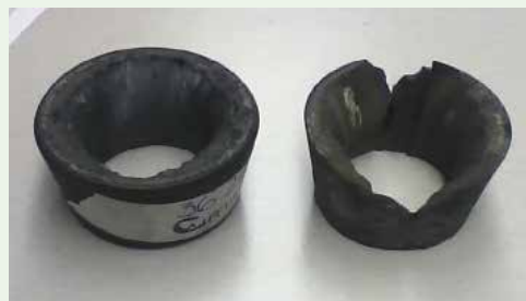
Comparison of recovered graphite throats. The throat on the left was flown with the new propellant formulation and shows less erosion than the throat on the right.
